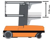
Material tray is electrically operated by a button in the upper control box
