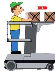
Loading platform at maximum height corresponds to the column. It is very easy to place even heavy packages using the column as the setting base and letting it slide into the material tray.
