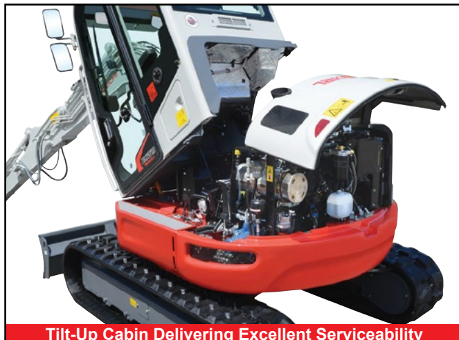
Tilt-Up Cabin Delivering Excellent Serviceability
