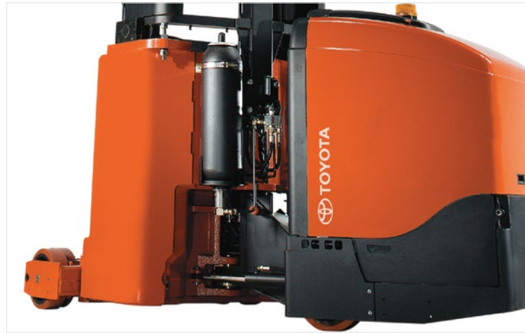
The A-series' Advanced Lifting System significantly reduces the amount of battery energy required to lift the cab and load, allowing two-shift operation on a single charge
