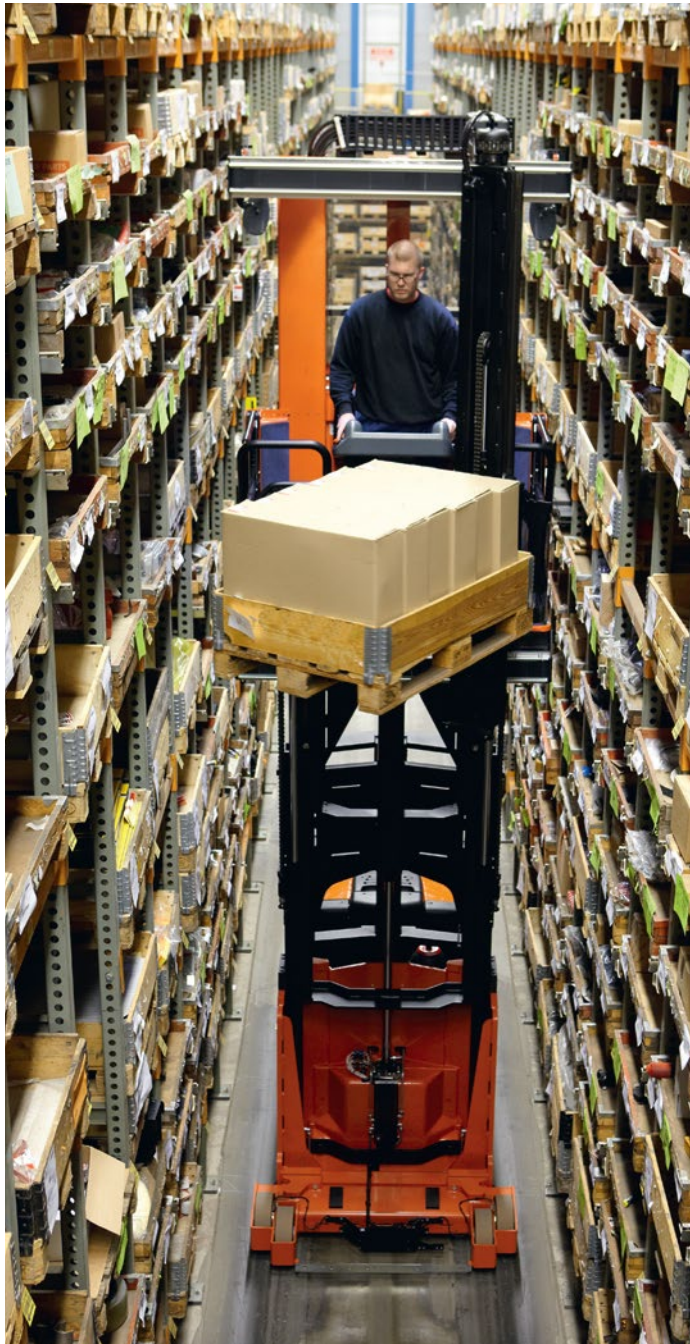
The A-series' Advanced Lifting System significantly reduces the amount of battery energy required to lift the cab and load, allowing two-shift operation on a single charge
